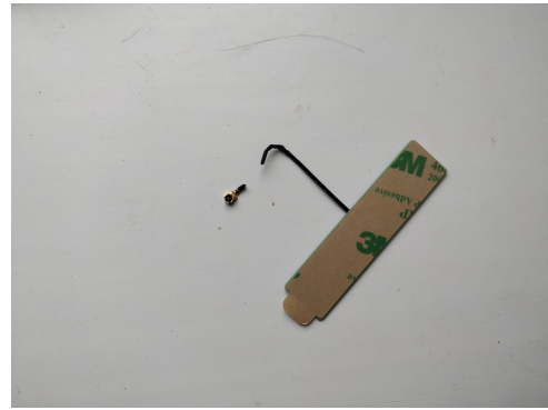
Figure 2.6: Damaged strip antenna.
